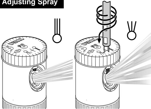
Turn the nozzle screw in to diffuse and shorten the spray radius.
